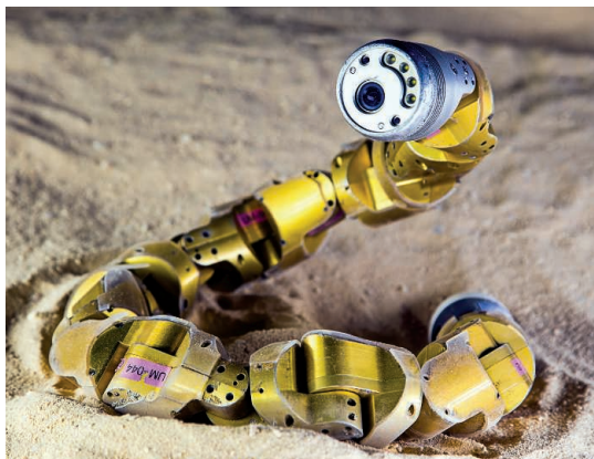
Sidewinding robot. By studying snakes and robots, Marvi et al. were able to elucidate how snakes sidewind and to modify a robot so that it could also achieve this feat.
